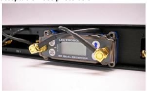
6. Power up the unit. Note that the power switch lights up green when the unit is turned on.
